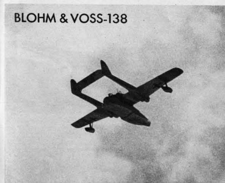
Odd-shaped hull gives BV-138 apt nickname "Flying Shoe." Used for reconnaissance, it was designed by the creator of asymmetrical BV-141.
